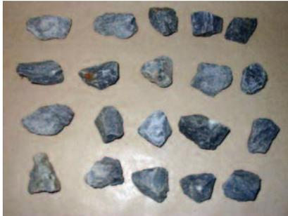
**Figure A1. Particles Selected for SMC Testing from Crushed Rock**
